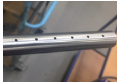
Fig. 8. New spray pipe for the drawing die spraying.
