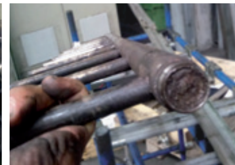
Fig. 4. Spray pipe of the drawing die clogged with copper sludge.
