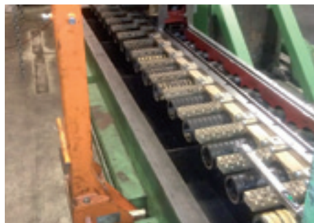
Fig. 2. Drawing area of the partially disassembled, cleaned and reconditioned MMH during reassembly.
