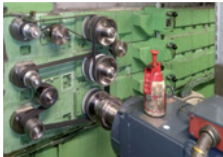
Fig. 6. Belt drive after reconditioning.
