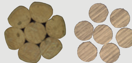
Fig. 4. Comparison of strands compacted with conventional technology (compacting before bunching) and with NIEHOFF “stretch forming and straightening” technology.
