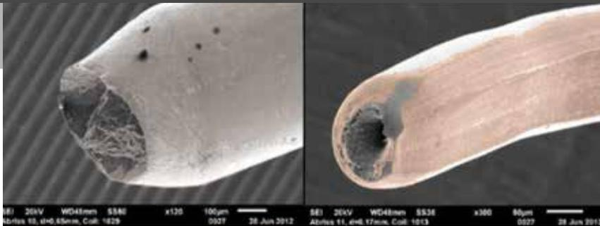
Fig. 1. The wire ends after a “cup-and-cone” break
