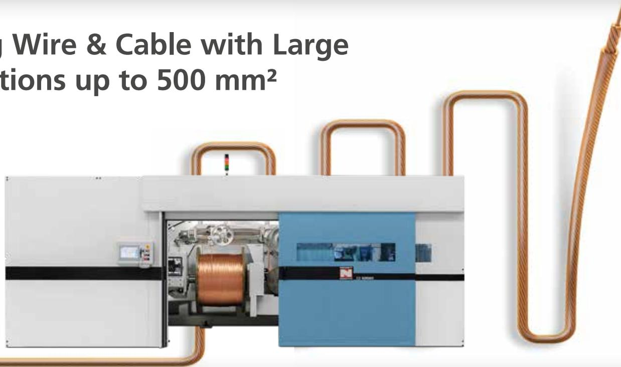
The new machine types **D 1252**, **D 1602** and **D 2002** for the production of conductors and conductor ropes for energy cables with cross sections between 6 and 500 mm<sup>2</sup> like all machines of the D series contain all crucial features modern bunching and stranding machines have to offer.
