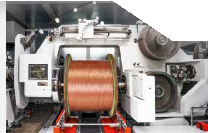
Fig. 4. Another characteristic is the energy-saving one bow design and the NBAT laying system
