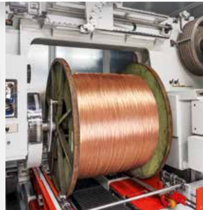
Fig. 3. The D 2002 accepts spools with a flange diameter of 2 m
